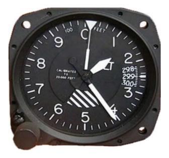
The long hand measures altitude in hundreds of feet ASL. This is the fastest moving hand of the three and a change in altitude will make it move.
